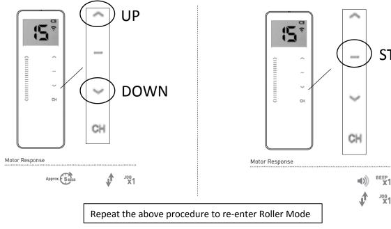
If you do not activate tilt mode in time the motor programming sequence will time out, repeat the above steps assuring to press the STOP button within 4 seconds of the motor jog
