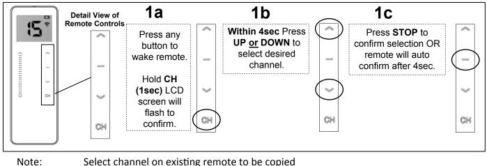
Select channel on existing remote to be copied Select channel on new remote where existing channel will be copied
