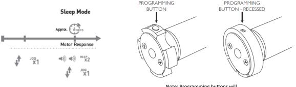
Note: Programming buttons will face down when shade is installed
