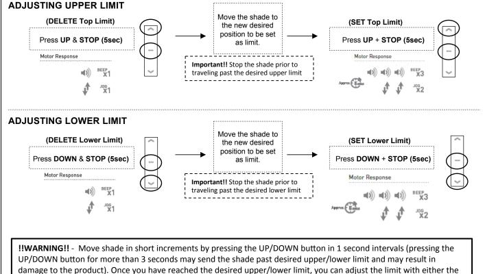
UP and DOWN buttons. (remember to adjust in short increments!)
