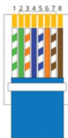
**RJ45 PINOUT T-568B**
