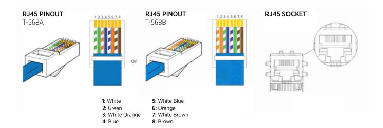
The standard connections of the Automate Pulse Hub 2 is Ethernet or WiFi. For a LAN connection, you can use a straight through wiring accordingly indicated above.
