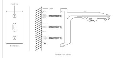
**3. Assemble Bracket:** Reassemble the brackets onto the backplates. Secure the brackets in place by tightening Hex screw on the bottom of the brackets.
