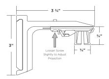
**7.** Once desired projection is set for all the brackets, lock the bracket into position by tightening the track depth adjustment set screw
