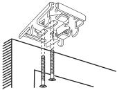
Hook the ridge of the headrail onto the back tab of the bracket as shown in the drawing below. Press locking tab on end and rotate headrail up to lock the headrail into place. Repeat this step for the remaining brackets.
