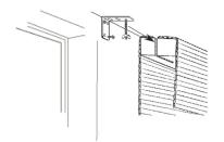
\* Please note that your brackets must be securely attached to the mounting surface. If your screws do not hit wood studs you'll have to use a different fastener which can be found at any local hardware store.
