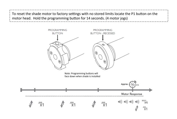
The motor will jog 4 times before the reset is complete. The P1 button must be held the entire time. 4 beeps confirm the factory reset is complete. Refer to the Initial Setup Programming section to program a shade after a factory reset.
