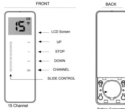
Battery Compartment (Shown with cover removed)
