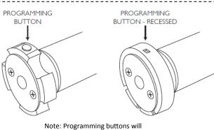
Note: Programming buttons will face down when shade is installed
