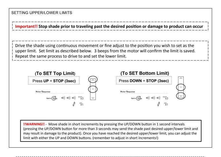
**Important!!** Remember to return the remote control to "L" mode as previously described to prevent inadvertent shade adjustment during normal operation and remote handling.
