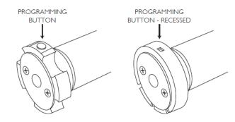
Note: Programming buttons will face down when shade is installed
