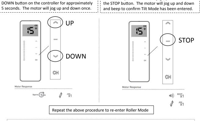
If you do not activate tilt mode in time the motor programming sequence will time out, repeat the above steps assuring to press the STOP button within 4 seconds of the motor jog
