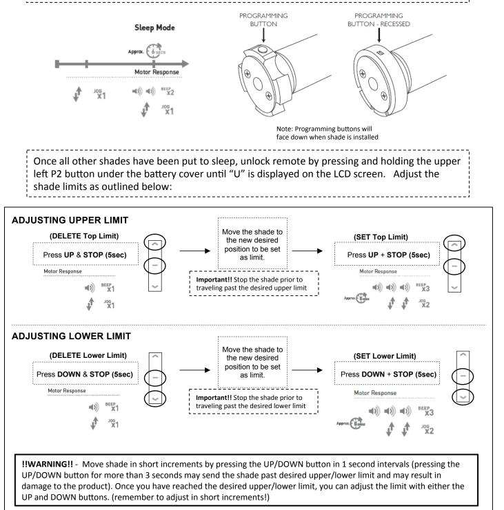
Once the limits have been adjusted as desired, return the remote control to "L" mode by pressing and holding the upper left P2 button under the battery cover. The other grouped motors can now be taken out of sleep mode by holding the programming button for 6 seconds
